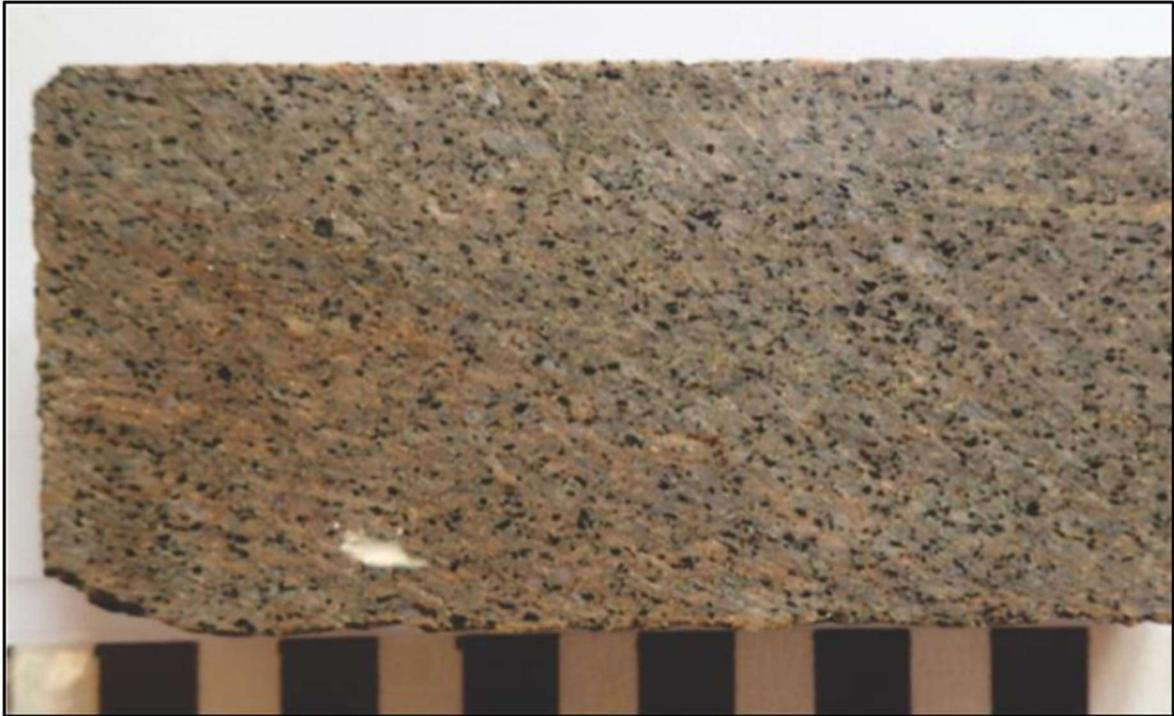
**Figure 12: Photograph of Metagranite in Core (Drill hole EC16-49).**
