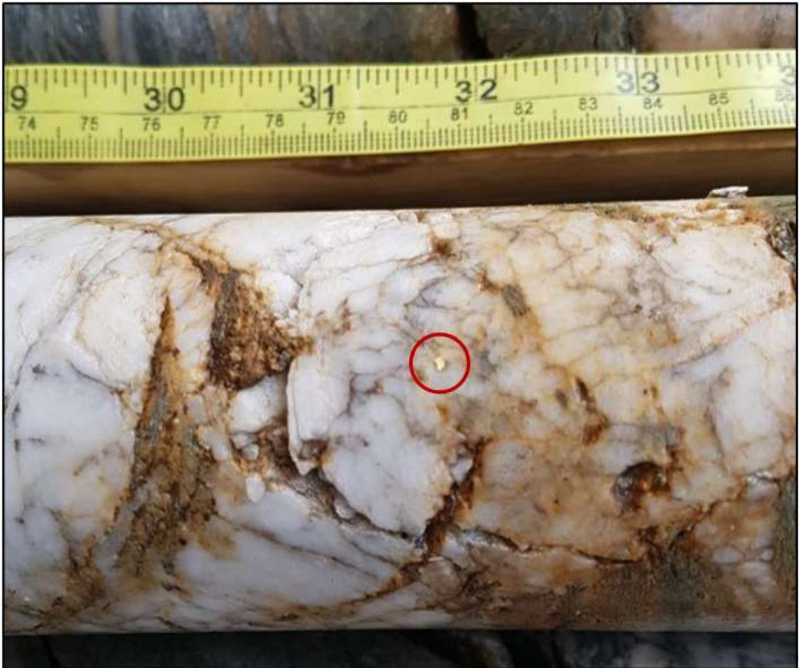
**Figure 15: Typical Cross-Cutting Quartz Vein with Native Gold Fleck from Drill Core (Hole LS20-350)**
