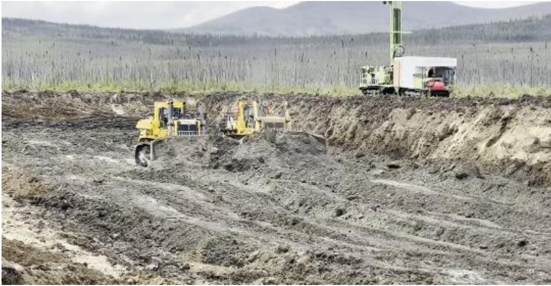
Figure 4: Stripping and work commencement at the Montana Creek Placer operation
