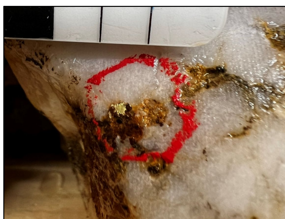
Figure 4c: Close-up photo of second visible gold grain in EC23-508 at 21.40m. Scale tick interval is 5mm.
