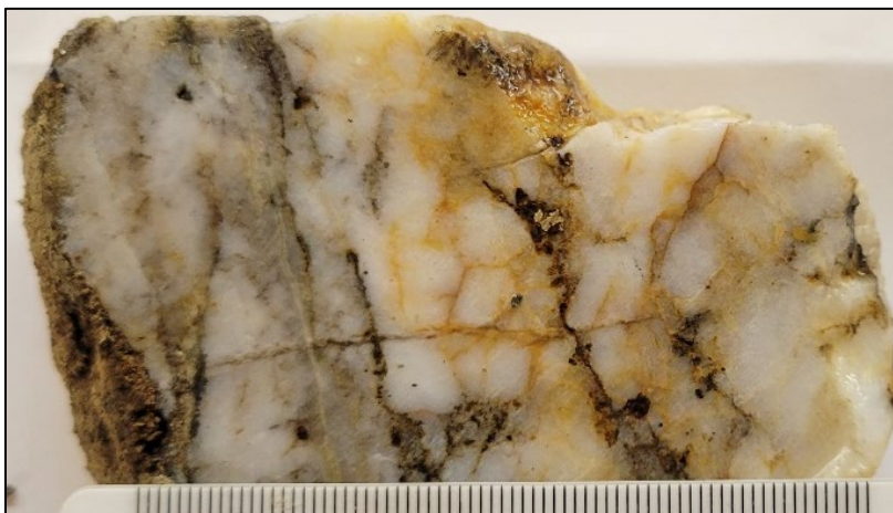
Figure 4a: Photo of quartz vein with visible gold in EC23-508 drill core interval at 21.34m. Scale ticks are 1mm.
