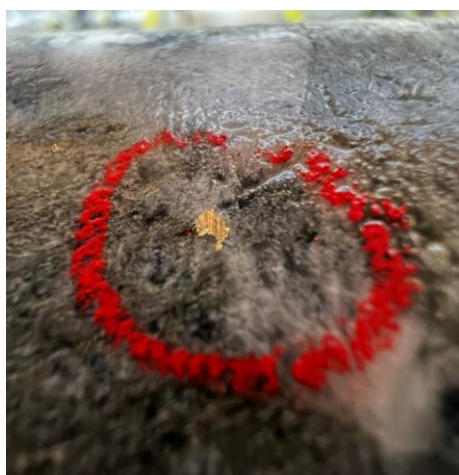
Figure 3: Photo of visible gold in EC23-503 drill core interval 111.97-112.18m: 12.90 g/t Au – within 0.38 g/t Au over 27.85m.
